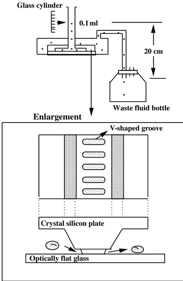
Fig. 2 Diagram of microchannel array flow analysis
