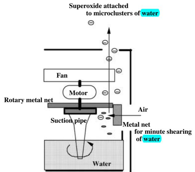
**Fig. 1** Diagram of water shearing appliance creating negative air ions. Water sucked via the rotary pipe jets out to the metal net and is then crushed minutely, when superoxide attached to microclusters of water is created
