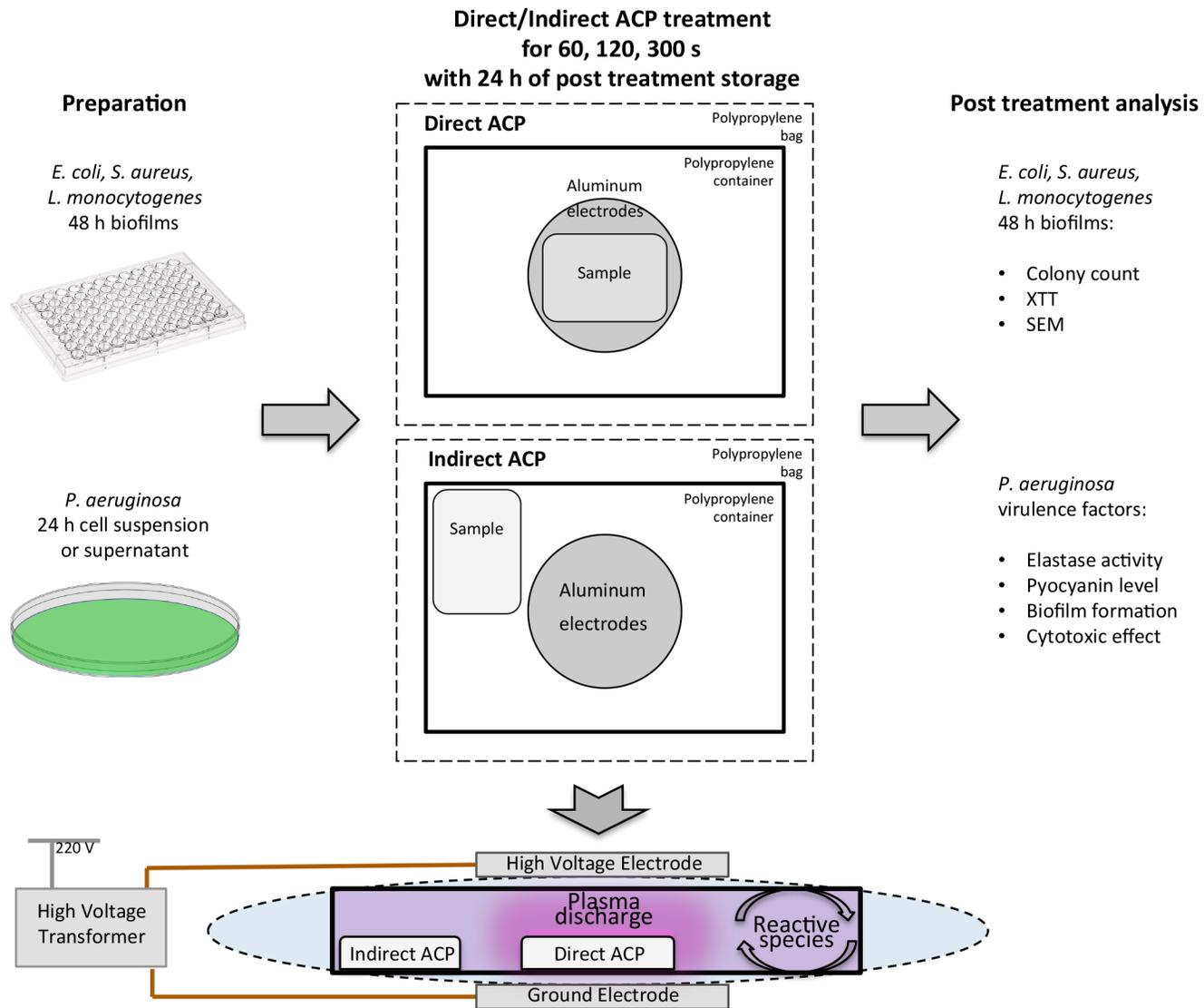
**Fig 1. Experimental set up.** Either a microtiter plate containing bacterial biofilms or a petri dish containing *P. aeruginosa* cells TSB suspension or cell-free supernatant were placed inside the plastic container between the electrodes for direct ACP treatment. For indirect ACP treatment, a separate container was used and samples were placed outside the plasma discharge.
