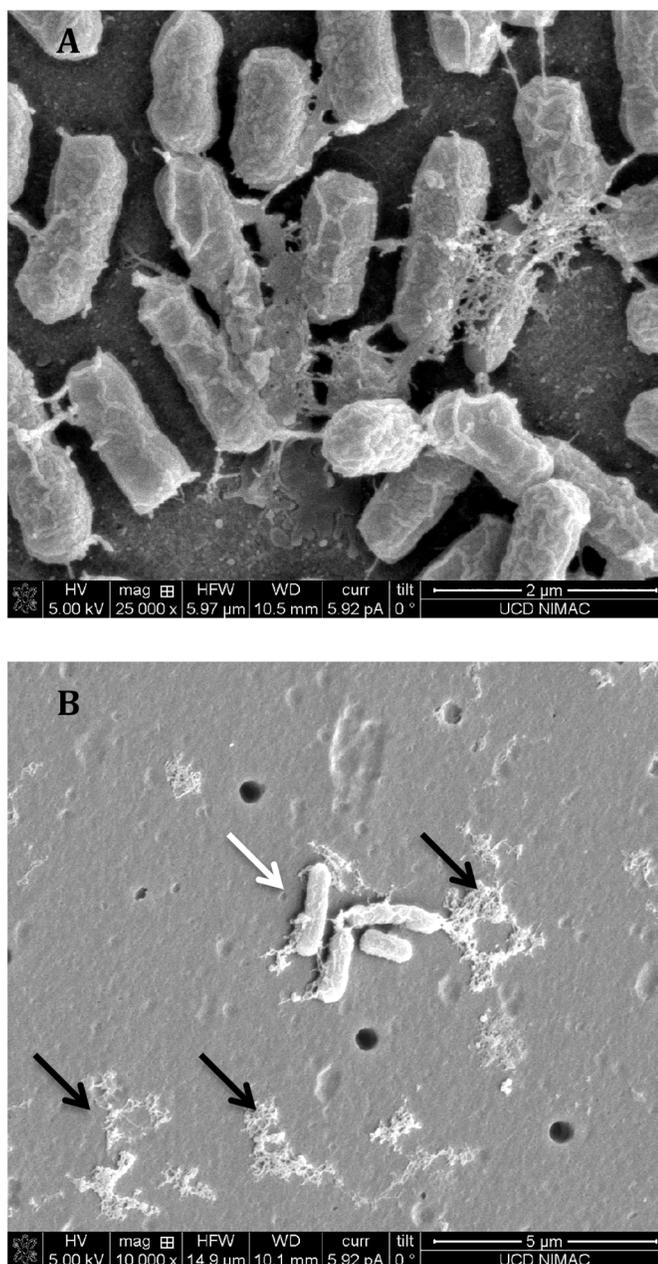
**Fig 4. Scanning electron microscopy images of *E. coli* 48 h biofilms.** (A) untreated 0 h control (magnification 25 000X) and (B) after 300 s of direct ACP treatment (magnification 10 000X). Black arrows indicate cell debris; white arrows indicate intact cells.
