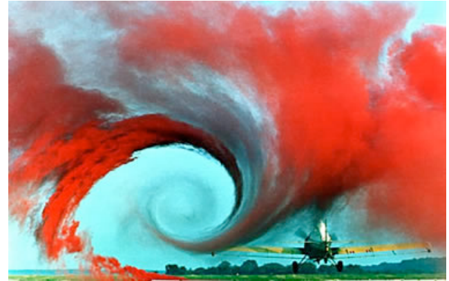
Turbulent flow (high Re)
