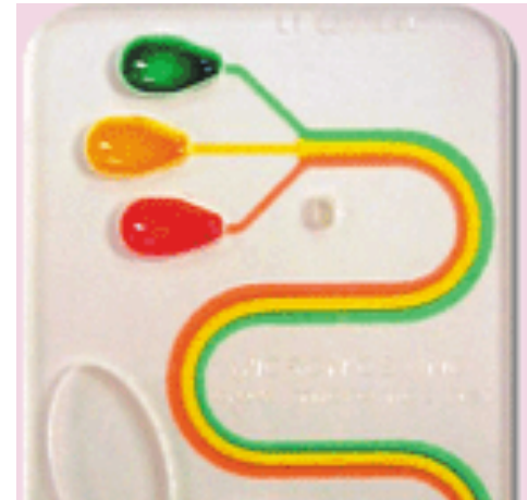
Laminar flow with orderly fluid motion (low Re)
